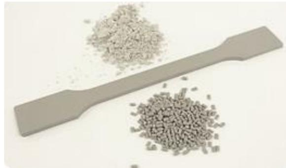
Figure 3. Wood Plastic Composite sample produced by VTT with the use of fly ash from the Utzenstorf mill
